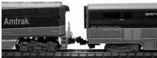
Out of the box , this locomotive demonstrates the result of a improperly installed clip and raised DCC pocket.
