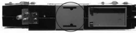
Figure 2: The holes in the top gray clip. These should be aligned towards the rear of the chassis as shown.
