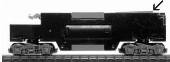
Figure 3: The raised DCC pocket (arrow). This should be filed flush with the chassis.
