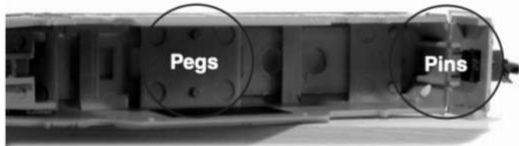
Figure 1 shows the pegs that insert in the clip on the chassis and the pins that hold the rear porch in place.
